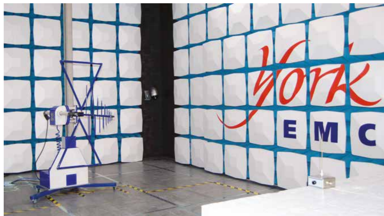
Figure 2. Radiated emissions pre-test check in operation
