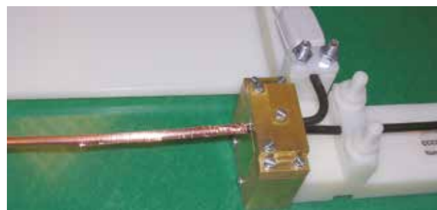
Figure 4. Injection strip fitted to Cable Under Test (CUT)
