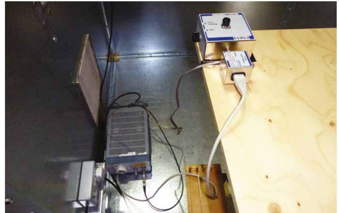
Figure 3. LISN verification setup using a CNE
