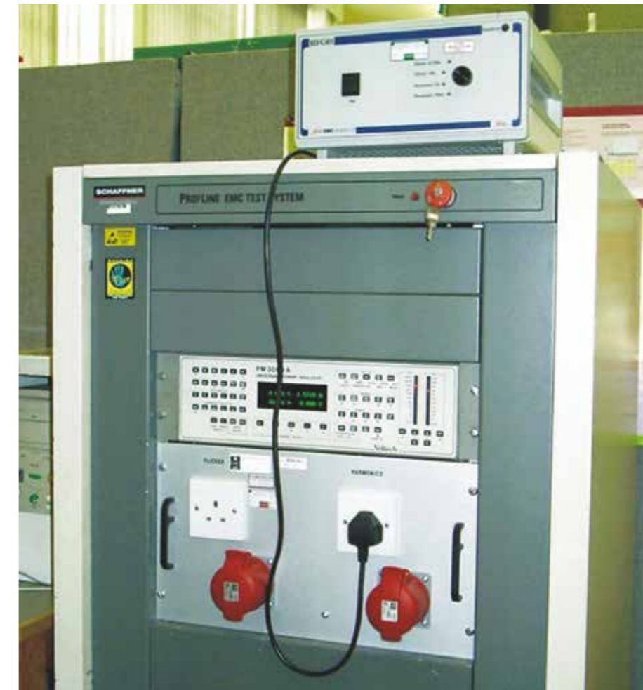
Figure 3. Harmonics pre-test using the HFG01 as the reference load
