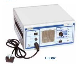
The HFG02 is a standalone device that connects directly to the test equipment and simulates the equipment under test (EUT), generating known, repeatable levels of harmonic and flicker disturbance.
