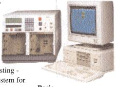
Basic ECAT® systems can simulate EFT, SURGE, PQF™ (Power Quality Failure) and ESD.
