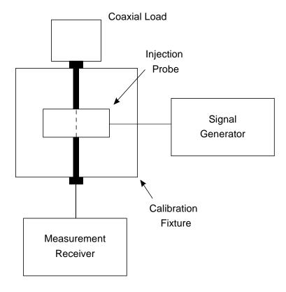
FIGURE A-11. Insertion loss measurement.
