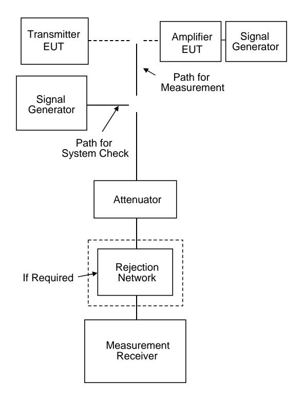
FIGURE CE106-1. Setup for low power transmitters and amplifiers.
