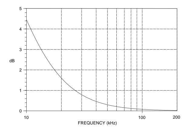
FIGURE A-4. Correction factor for LISN capacitor.
