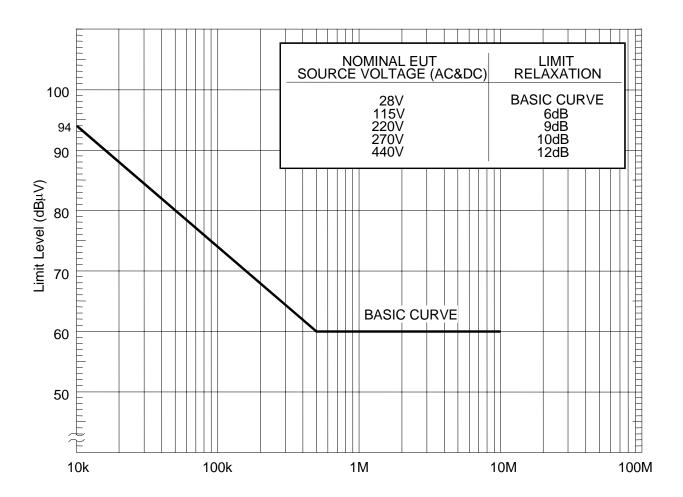
FIGURE CE102-1. CE102 limit (EUT power leads, AC and DC) for all applications.
