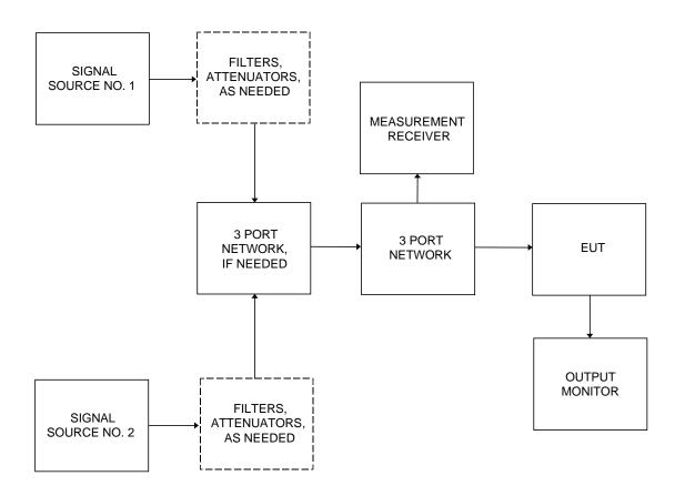
FIGURE A-8. CS105 General test setup.
