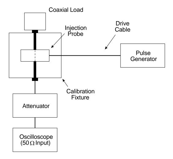
FIGURE CS115-2. Calibration setup.
