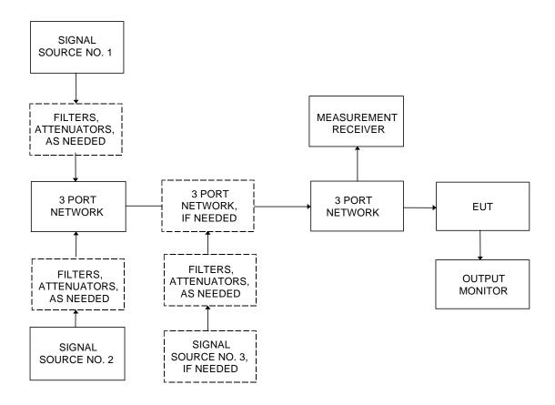
FIGURE A-6. CS103 General test setup.
