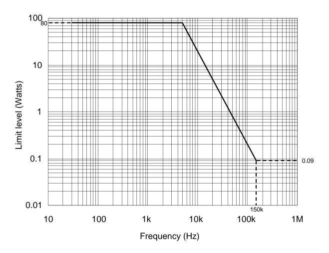
FIGURE CS101-2. CS101 power limit for all applications.
