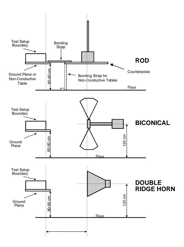
FIGURE RE102-6. Antenna positioning.
