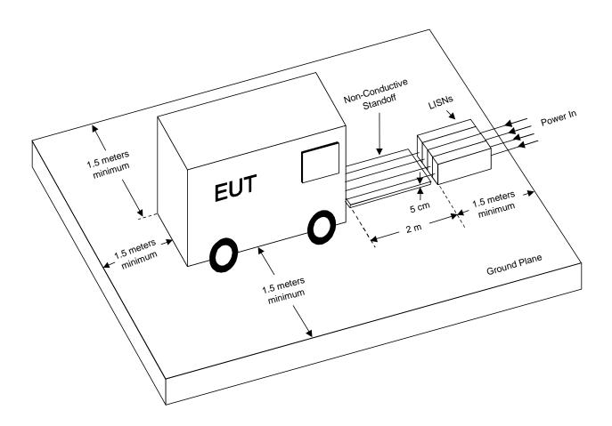
FIGURE 5. Test setup for free standing EUT.
