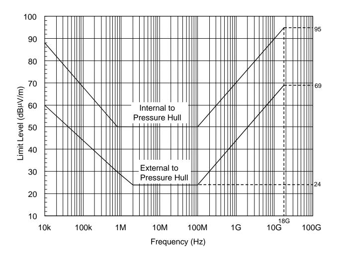
FIGURE RE102-2. RE102 limit for submarine applications.
