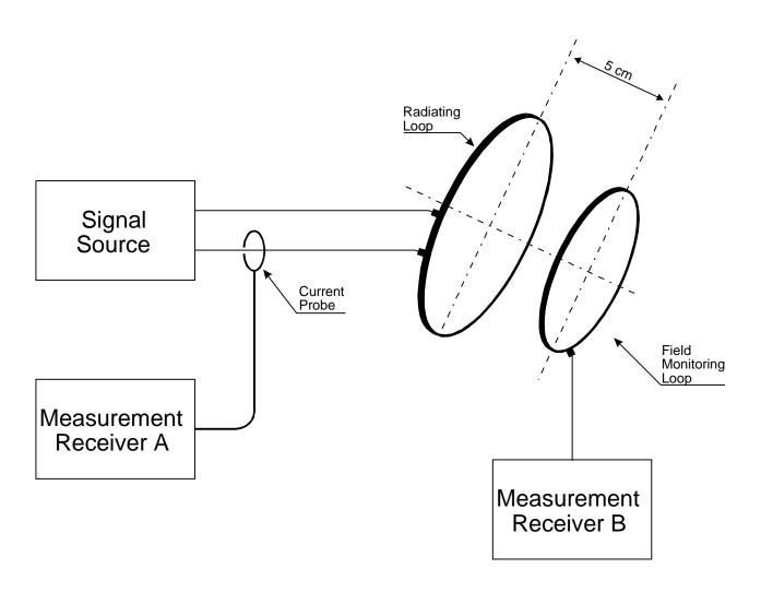
FIGURE RS101-3. Calibration of the radiating system.
