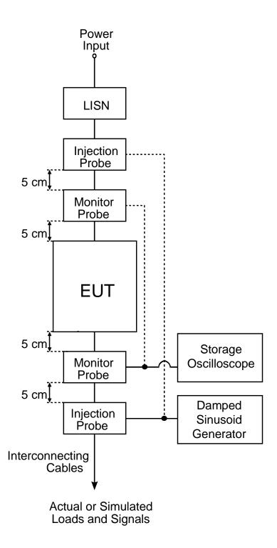
FIGURE CS116-4. Typical set up for bulk cable injection of damped sinusoidal transients.
