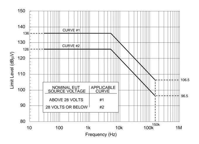
FIGURE CS101-1. CS101 voltage limit for all applications.
