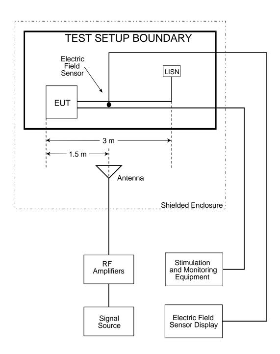
FIGURE RS103-1. Test equipment configuration.
