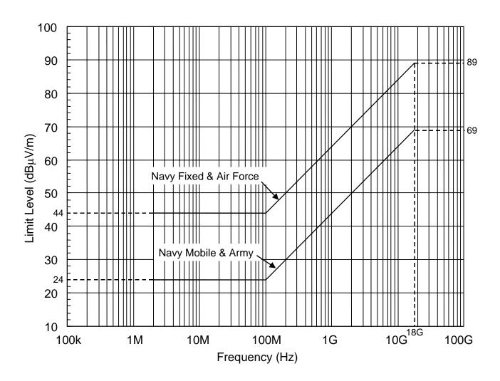
FIGURE RE102-4. RE102 limit for ground applications.
