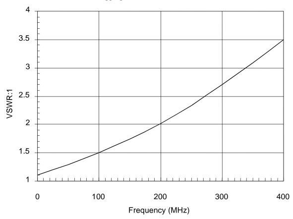
FIGURE A-10. Maximum VSWR of calibration fixture.
