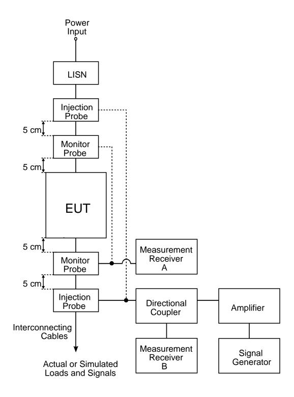
FIGURE CS114-4. Bulk cable injection evaluation.
