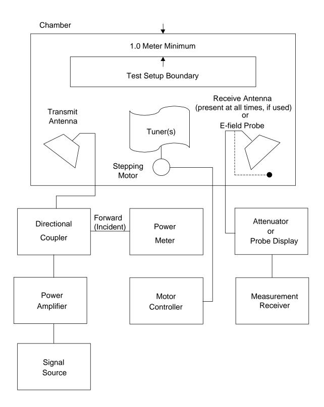
FIGURE RS103-5. Reveberation chamber setup.
