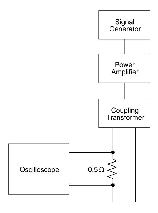
FIGURE CS101-3. Calibration.
