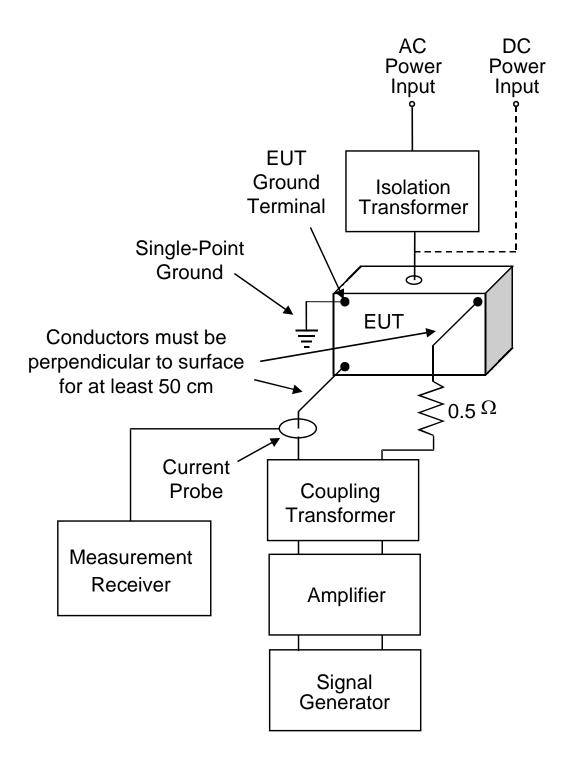
FIGURE CS109-2. Test Configuration.
