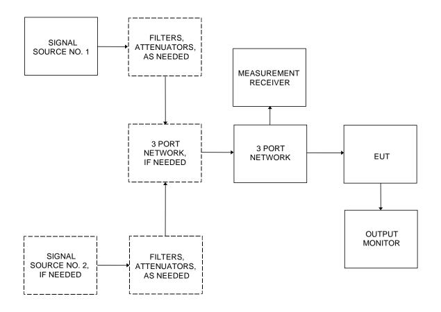
FIGURE A-7. CS104 General test setup.
