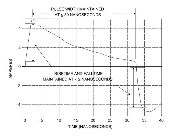
FIGURE A-13. Typical CS115 calibration fixture waveform.
