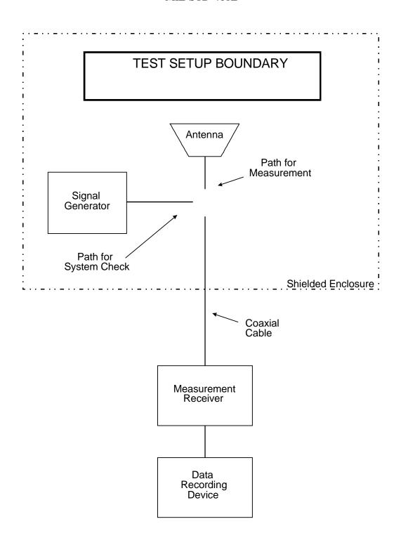
FIGURE RE102-5. Basic test setup.
