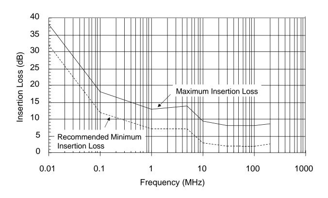
FIGURE CS114-2. Maximum insertion loss for injection probes.
