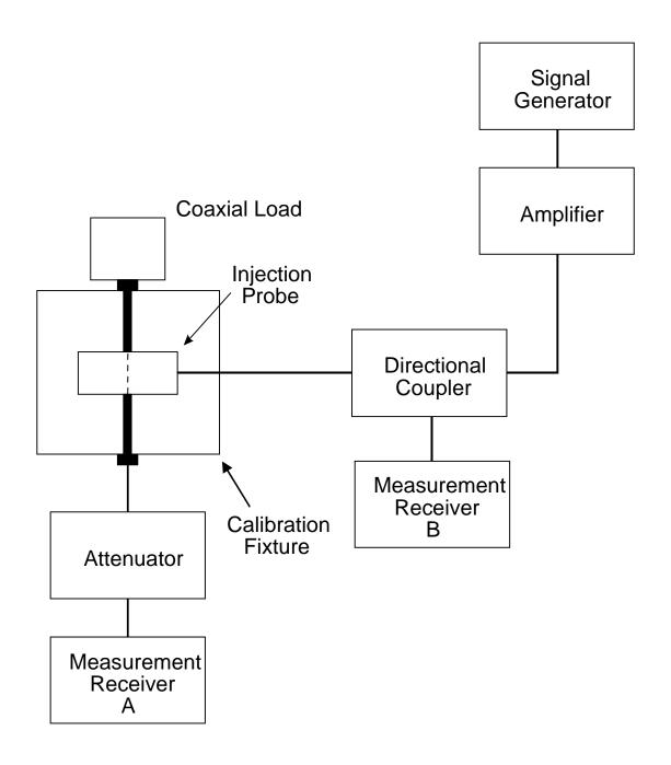
FIGURE CS114-3. Calibration setup.
