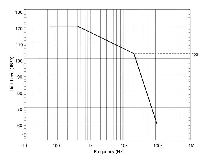
FIGURE CS109-1. CS109 limit for all applications
