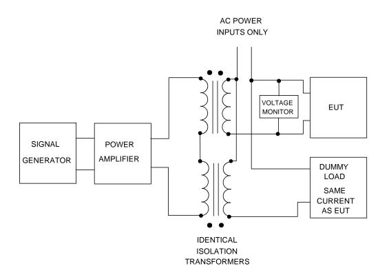
FIGURE A-5. CS101 Power amplifier protection.
