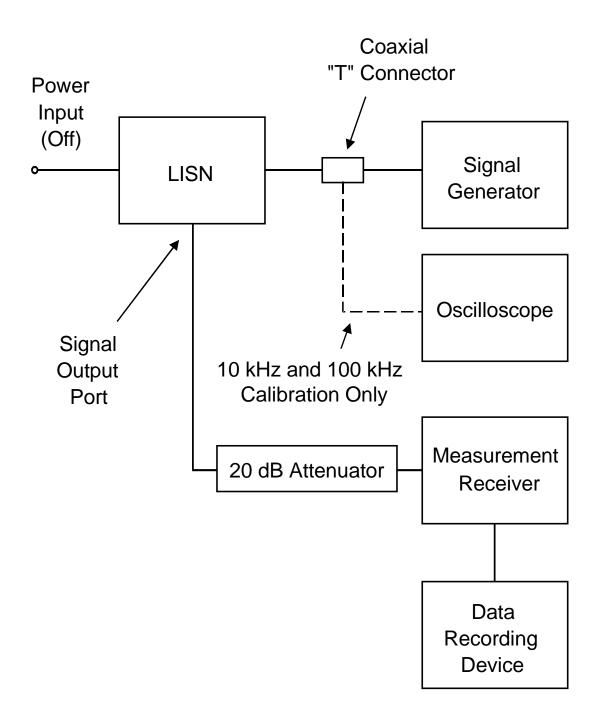
FIGURE CE102-2. Measurement system check setup.
