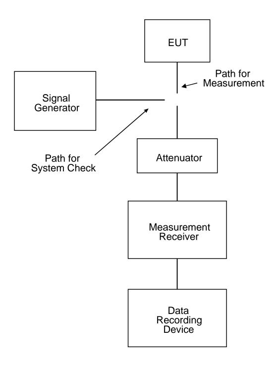
FIGURE CE106-3. Setup for receivers and stand-by mode for transmitters and amplifiers.
