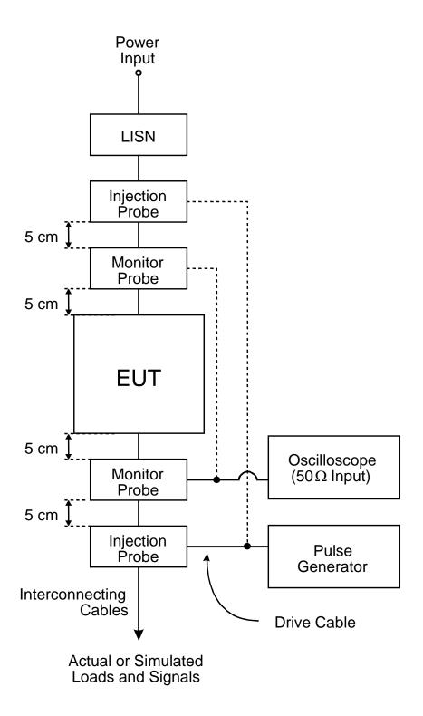
FIGURE CS115-3. Bulk cable injection.
