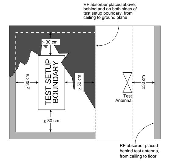
FIGURE 1. RF absorber loading diagram.
