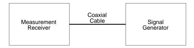
FIGURE RE101-3. Calibration configuration.
