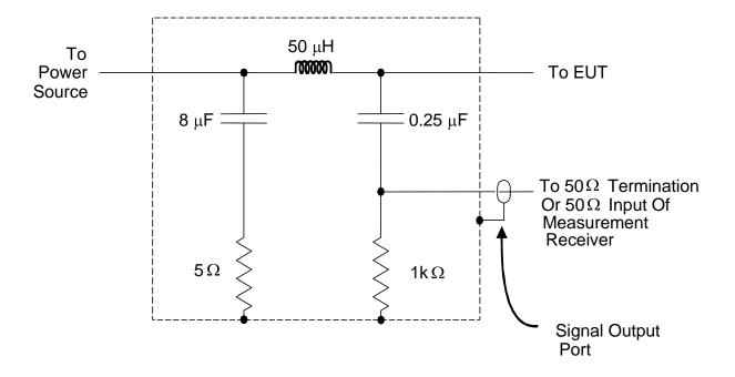
FIGURE 6. LISN schematic.
