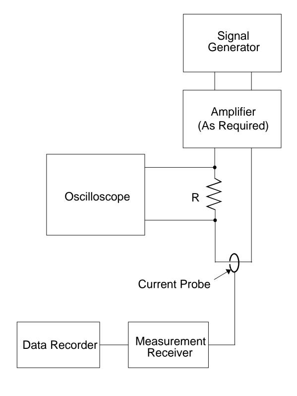
FIGURE CE101-5. Measurement system check.
