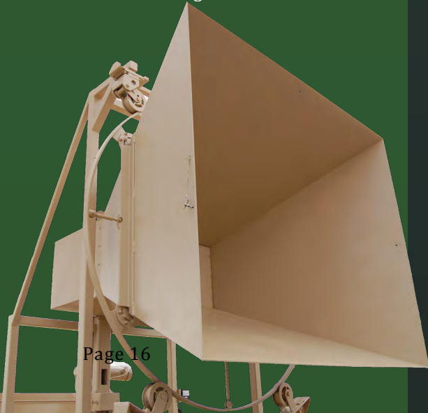
TMC Design's newest antenna trailer, the HO-4925-13 Horn Antenna, operates in the 150 to 229 MHz range
