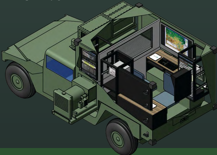
A forward deployable, mobile SSA concept utilizing a HMMWV shelter
