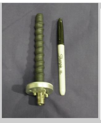
The HE-0580-10 is a high power, right hand circularly polarized (RHCP) severe duty small antenna for both military and commercial applications. The antenna is constructed entirely of aircraft certified 6061-T6 aluminum and G-10 fiberglass with copper radiator in a 100% sealed radome. This antenna was custom matched from 5.0 to 6.0 **GHz** to have the lowest VSWR possible, achieving a 2: 1VSWR across the band. The antenna is designed to provide many years of service.
