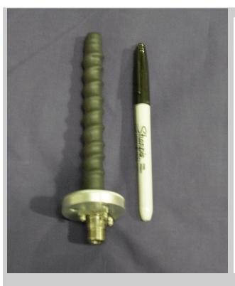
The HE-0075-10 is a high power, circularly polarized (RHCP or LHCP) severe duty physically small antenna for both military and commercial applications. The antenna is constructed entirely of aircraft certified 6061 -T6 aluminum and G-10 fiberglass with copper radiator in a 100% sealed radome. This antenna is custom matched from 4.0 to 5.0 GHz to have the lowest VSWR possible, achieving a 2:1 VSWR across the band. The antenna is designed to provide many years of service.
