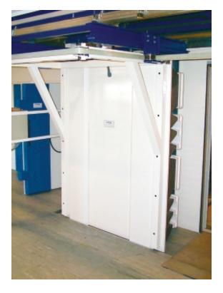
The TDK Sliding Doors combine industrial quality construction with high-performance absorber materials to provide fully automatic operation and excellent RF-shielding.
