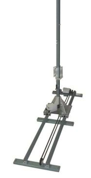
The TDK PP-02 Field Probe Positioner permits remote x-y positioning in EMC test environments. The PP-02 supports field uniformity schemes as well as flexible grid definitions for a variety of test requirements.
