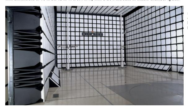
10 meter test range semi-anechoic chamber constructed by TDK utilizing **IP-090BL** absorbers.
