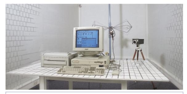
**IB-015** ferrite tile absorbers in a TDK CAC-R compact anechoic chamber (white painted finish is optional).
