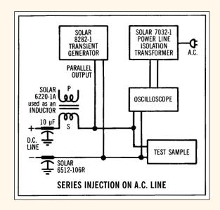
**Power Current in Series Injection Mode:** Handles up to 50 amperes of current at power frequencies.
