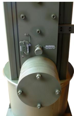
Elevation axis locked
