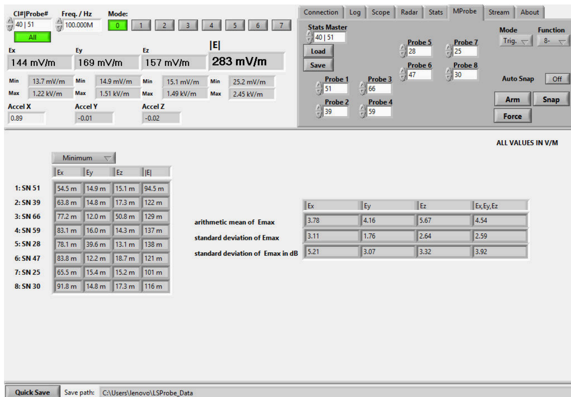
Figure 34: LSProbe GUI, Multiprobe tab for eight probe setups
