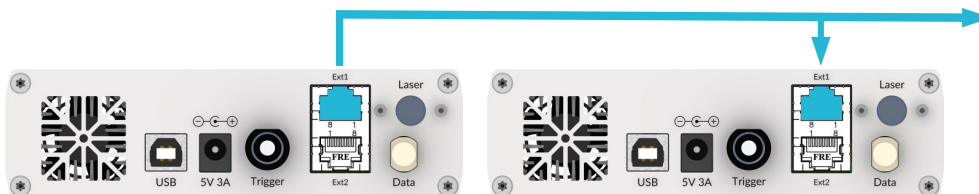
Figure 13: External trigger input and output using Ext1 RJ45 sockets
