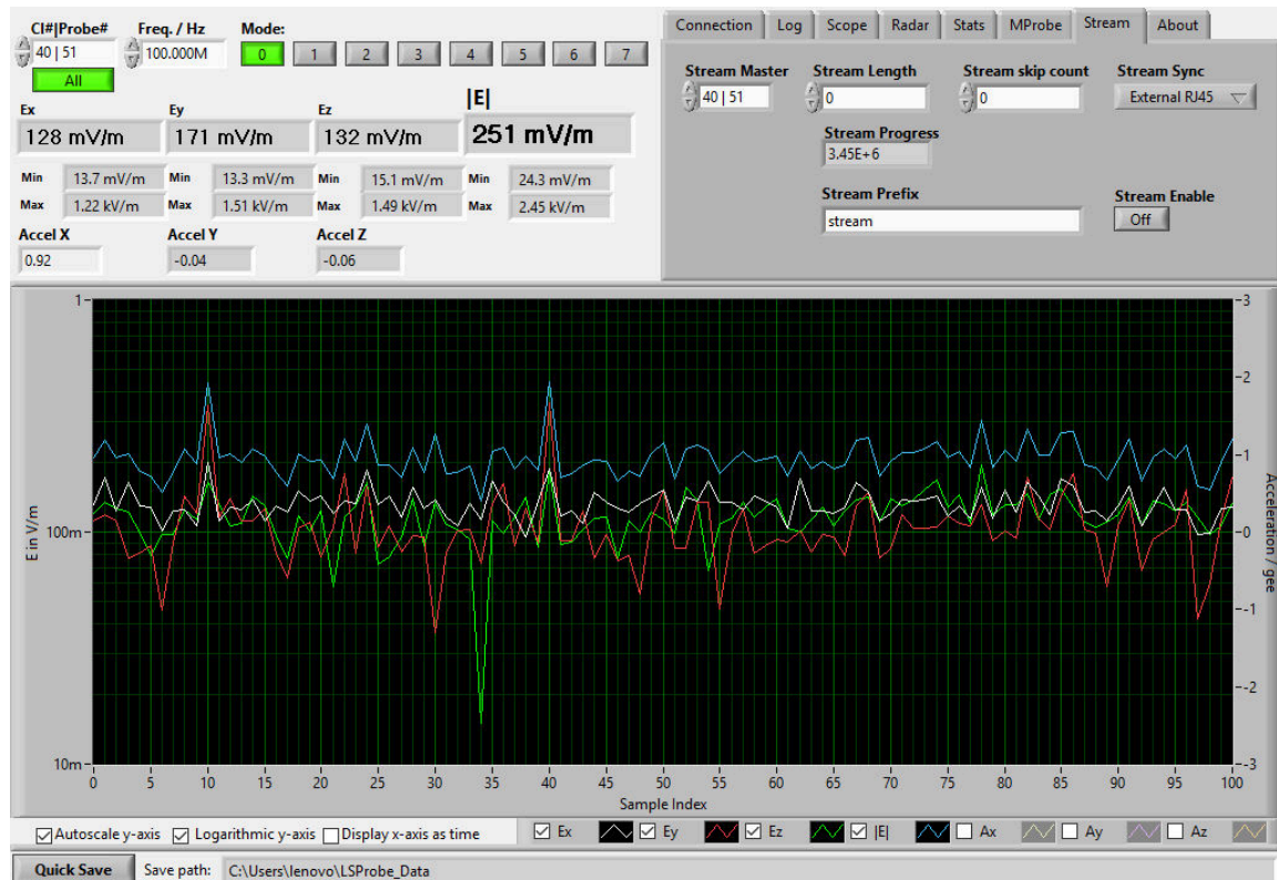
Figure 36: LSProbe GUI, Stream tab for stream recording
