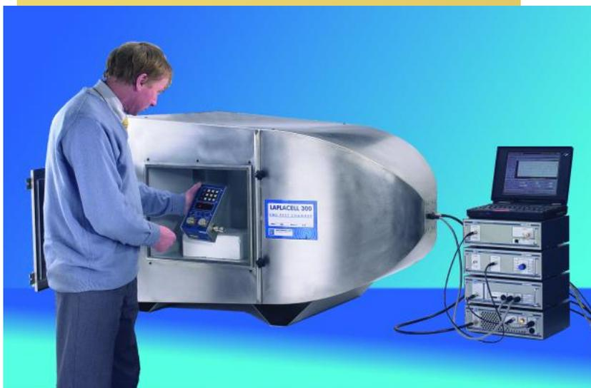
The LaplaCell is a unique concept featuring a balanced seipum design, proven to deliver better uniformity of field than any other GTEM or similar compact cell.
