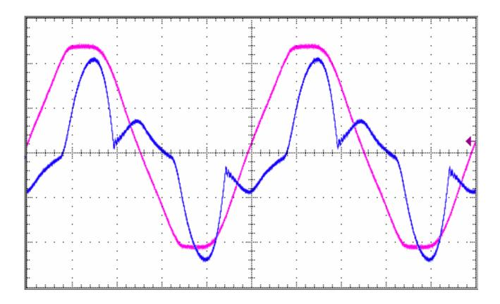
The figure shows a typical mains voltage waveform as available at a normal socket outlet. The flat top distortion is clearly evident; this shows the effect on the supply network of harmonic currents caused by large numbers of electronic products taking a sharply peaked current waveform such as that illustrated.
