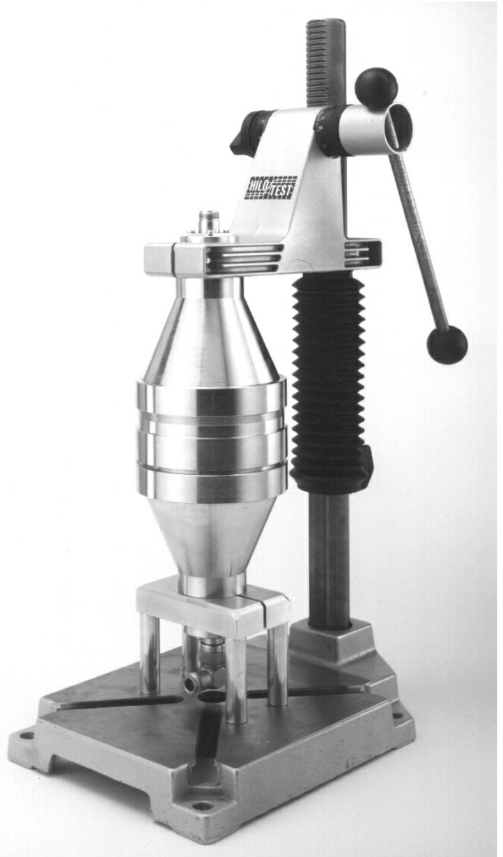
The TEM – Measuring Cell TEM -2000 permits the measurement of the screening attenuation of electrical conducting plastics, conducting laminated plastics, screening materials and braids.
