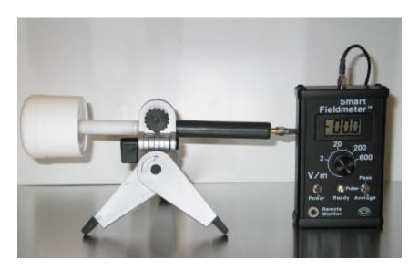
Smart Fieldmeter™ can be used for RF Radiated Immunity testing for practically any EMC standard, including MIL STD 461/462, RTCA DO-160, EN50082, EN61000-4-3, etc.).
