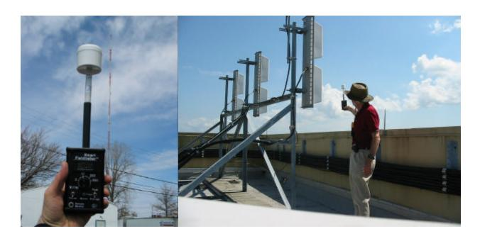
Smart Fieldmeter™ can be used for evaluation and measurements of EM fields from various field sources: AM/FM/TV and cellular stations; transmitters and CB radios, etc. Its multimode (Average, Peak and Pulse) operation allows monitoring of the steady state and pulsed fields by displaying the average or peak values.
