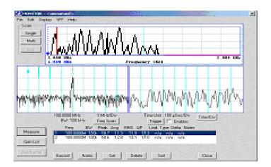
**Time Domain Display:** the right center panel shows an oscilloscope type display of the detected signal. Variable time- base and trigger controls are available.
