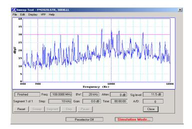
The DSI-2020 gives the user full control, even during the automated sweep. The sweep can be "paused" to investigate signals of interest and resume at any time. The sweep can proceed one step at a time, and a logical mode permits manual control of the receiver for investigative work.
