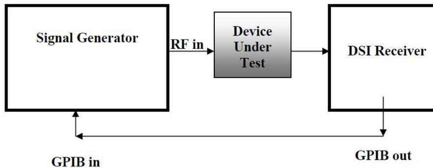
Figure 3. Swept frequency tracking with a DSI Receiver
