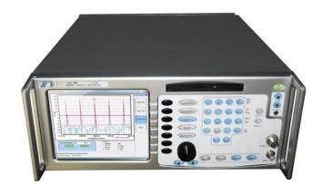
The DSI-600 state-of-the-art super heterodyne receiver operates from 20 Hz to 40 GHz. Highly specialized for both MIL-STD and CISPR Compliance testing.
