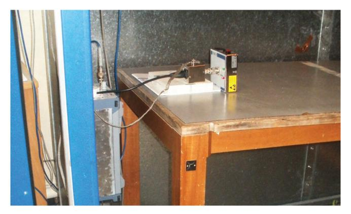
Figure 3. LISN verification setup using a CNE
