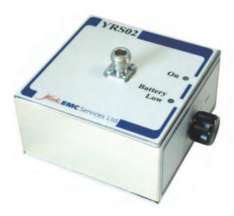
For radiated operation, antennas can be attached to the unit's output connector. Two monopole antennas, optimised for different frequency bands, are available. The YRS02 is an ideal source for carrying out checks on open area test sites (OATS) and anechoic chambers.
