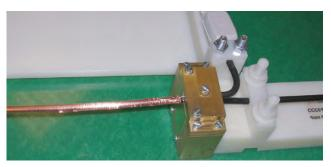
Figure 4. Injection strip fitted to Cable Under Test (CUT)
