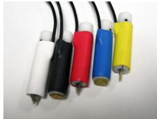
H Field, E Field and direct injection probes used for susceptibility scanning Courtesy of Amber Precision Instruments
