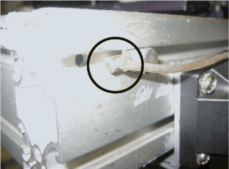
Figure 1. Broken Grounding Wire
