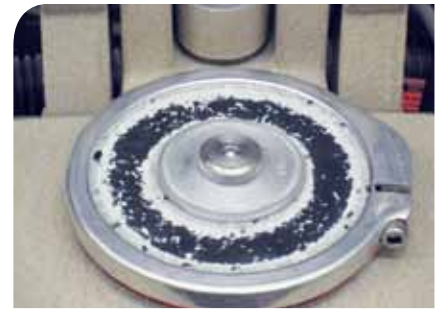
Rubber tile: After 3,000 abrasion cycles, the conductive layering was nearly all worn away, exposing the black rubber below.
