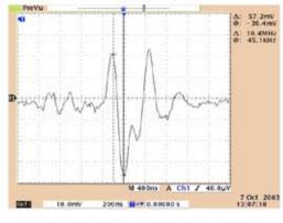
Figure 2a. Current in GBB (gold ball bonding) Tool (peak current is 182mA)
