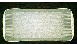
EOS Damage of Capacitor Source: Assurance Technology
