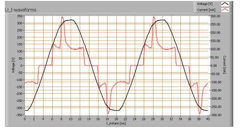
A typical waveform of mains signal from UPS. This signal contains very significant harmonics that gets induced on ground
