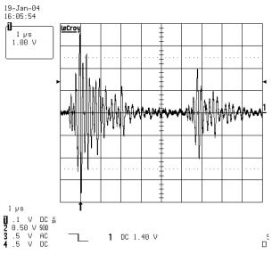
Figure 3. Voltage between the tip of a tool and ground. Peak voltage is ~3.6V
