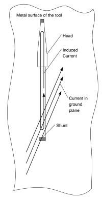
Figure 6. Inductive Coupling Between Ground Current and the Head
