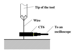
Figure 4. Current Measurement Setup in the Tool
