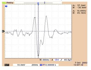
Figure 5. Current in GBB (gold ball bonding) Tool (peak current is 182mA)
