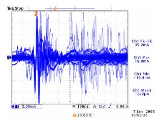
Figure 7. Current induced by transformer coupling in the tool (peak value – 35mA). Multiple signals are often present on ground as seen.
