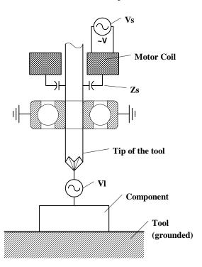
Figure 2. Generation of Voltage in a Tool via Capacitive
