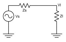
Figure 1. Basic Voltage Source
