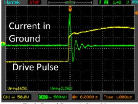
Fig. 8 Ground Current in Servo Motor
