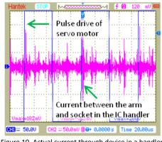
Figure 10. Actual current through device in a handler
