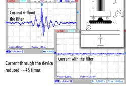
Figure 14. Reduction of EOS current using SF-series filter
