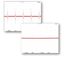
Figure 13. Ground current without and with SF filter
