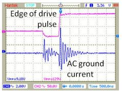
Figure 7. AC ground current caused by operation of a
