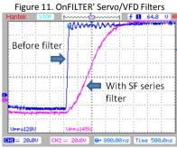
Figure 12. Typical edge modification of servo drive signal by a SF series filter
