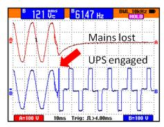
Figure 4. Switchover to UPS Source: Repeater-Builder
