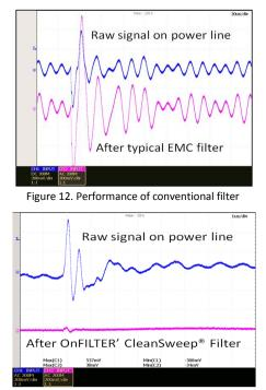
Figure 13. Performance of CleanSweep<sup>®</sup> filter
