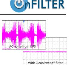
Figure 9. CleanSweep<sup>®</sup> filter reduces output transients from UPS
