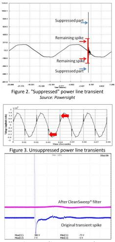
Figure 4. CleanSweep filter suppression performance
