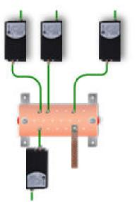
Figure 6. Connection of ground line filters GLE30 to a ground bar
