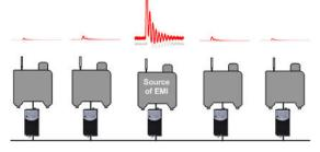
Figure 3. Ground filters GLE30-1 block propagation of EMI
