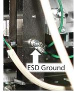
Figure 2. Typical ESD grounding inside the tool
