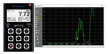
The user can, by way of a mouse, highlight a portion of the graph and automatically focus on the corresponding readings or measurements within that area in a tabular format.
