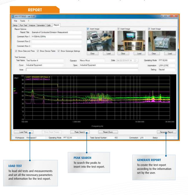
**FFT 3030 EMI Receiver** is ideally suited for measurement of electromagnetic interference in accordance with the requirements of CISPR 14-1 (household appliances industry) and CISPR 15 (lighting equipment industry) standards.
