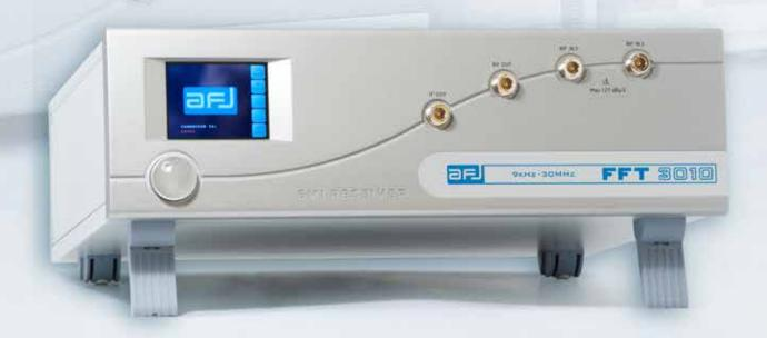
Compact designed and manufactured compliant to CISPR 16 International Standard, using FFT Scan Mode for fast measurements of conducted electromagnetic interference in accordance with requirements of EMI International, European and Product standards, pre-selectors and advanced software for EMC testing.
