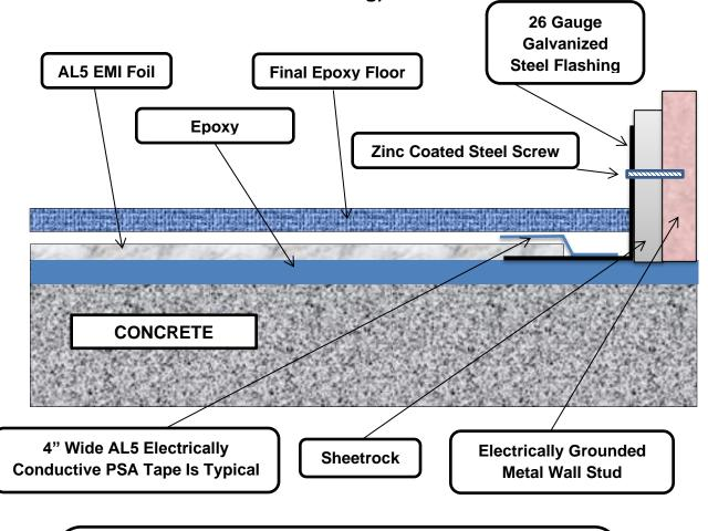
4" x 4" or 6" x 6" 26 Gauge Galvanized Steel L Flashing is Typical
