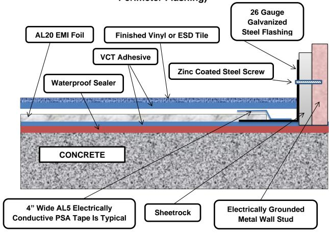
4" x 4" or 6" x 6" 26 Gauge Galvanized Steel L Flashing is Typical Wall Shielding Attaches to the Vertical Portion of the Flashing Clear Zinc Coated Screw Anchors in to the Metal Wall Stud to
