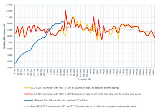
AL5 EMI foil shielding is applied like wallpaper, covering all surfaces: floor, walls and ceiling. Other than normal cleanliness, and dust free, no special preparation is required. Raw sheetrock will be required to be primed if you are using the AL5 with PSA. The foil should be glued in-place or ordered with a Pressure Sensitive Adhesive (PSA).
