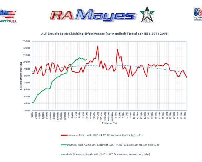
**AL5** EMI foil shielding is applied like wallpaper, covering all surfaces: floor, walls and ceiling. Other than normal cleanliness, and dust free, no special preparation is required. Raw sheetrock will be required to be primed if you are using the AL5 with PSA. The foil should be glued in-place or ordered with a Pressure Sensitive Adhesive (PSA).
