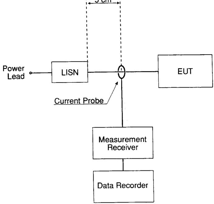
FIGURE CE101-2. Measurement setup.
