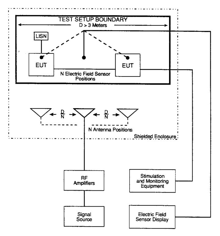
FIGURE RS103-3. <u>Multiple test antenna locations for</u> <u>N positions, D > 3 meters</u>.
