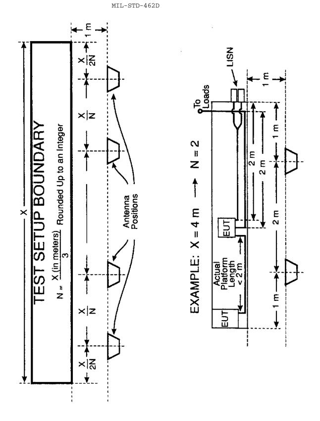
FIGURE RE102-3. Multiple antenna positions.
