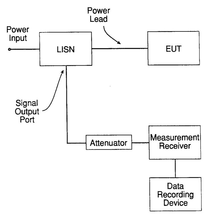
FIGURE CE102-2. Measurement setup.
