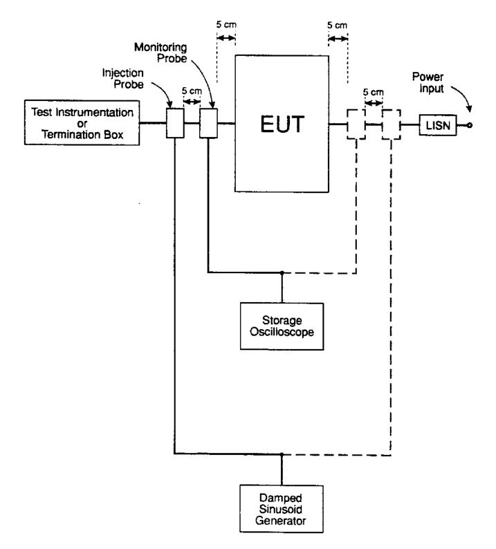
FIGURE CS116-3. <u>Typical set up for bulk cable injection</u> of damped sinusoidal transients.
