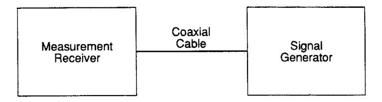
FIGURE RE101-2. <u>Calibration configuration</u>.
