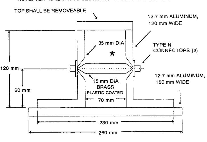
NOTE: VERTICAL CROSS-SECTION AT CENTER OF FIXTURE SHOWN
