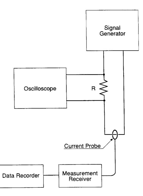
FIGURE CE101-1. Measurement system check setup.
