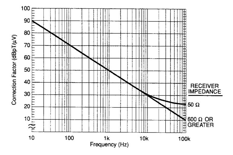
FIGURE RE101-1. Loop sensor correction factor.
