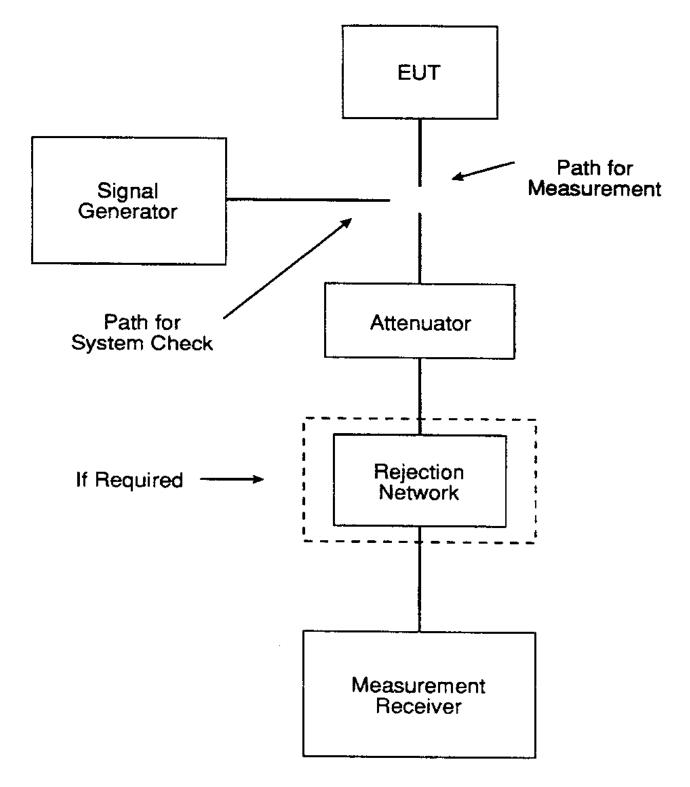
FIGURE CE106-1. Setup for low power transmitter.
