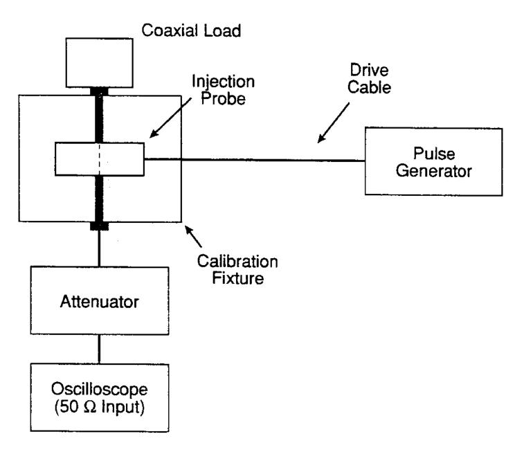
FIGURE CS115-1. <u>Calibration setup</u>.
