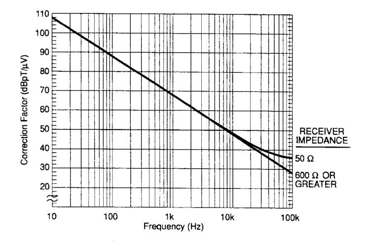
FIGURE RS101-1. Loop sensor correction factor.
