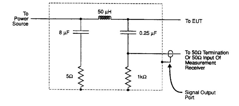
FIGURE 6. LISN schematic.
