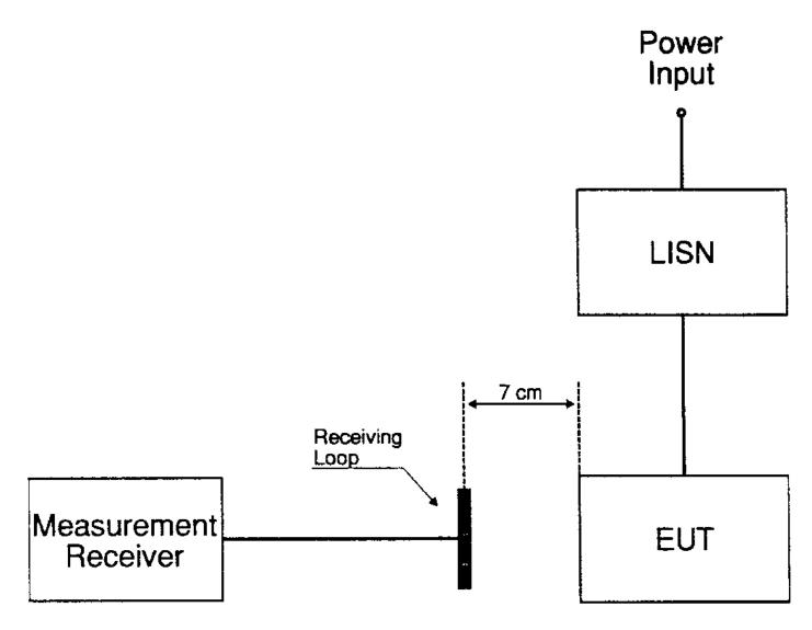
FIGURE RE101-3. <u>Typical Test Setup for Radiated</u> <u>Emissions, Magnetic Field, 30 Hz to</u> <u>100 kHz</u>.
