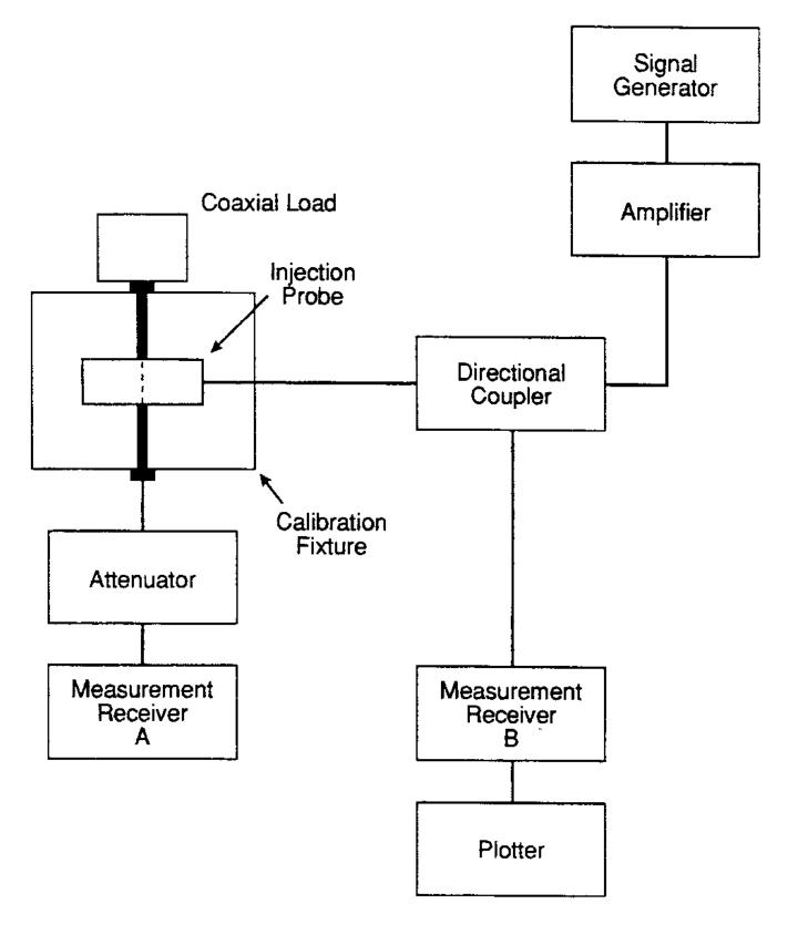
FIGURE CS114-1. <u>Calibration setup</u>.
