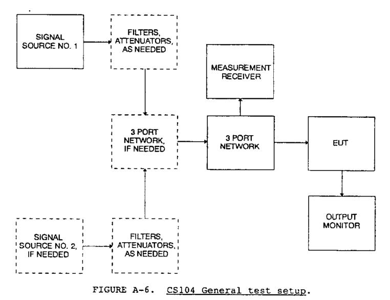
Typical data for this test method for the EMITR are the sensitivity of the receiver, the levels of the signal sources, frequency ranges swept, operating frequencies of the receivers, degree of rejection (dB), and frequencies and threshold levels associated with any responses.
