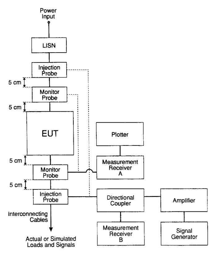
FIGURE CS116-2. Loop circuit impedance characterization.
