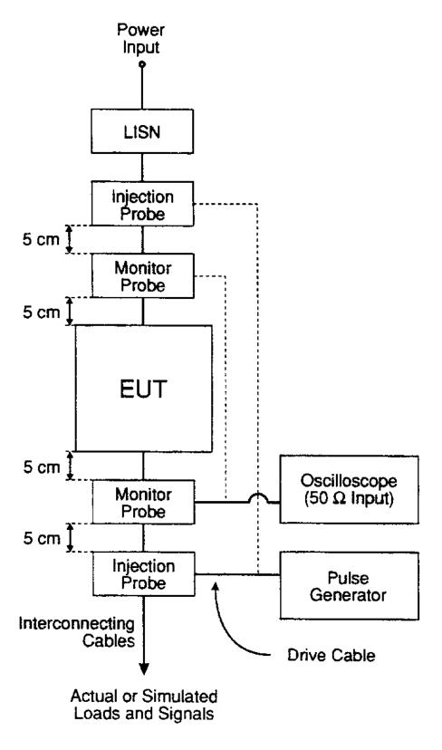
FIGURE CS115-2. Bulk cable injection.
