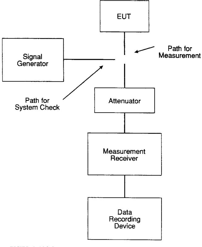
FIGURE CE106-3. <u>Setup for transmitters (stand-by mode)</u> and receivers.
