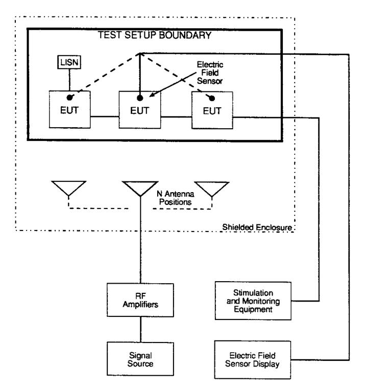
FIGURE RS103-2. <u>Multiple test antenna locations for</u> <u>frequency > 200 MHz</u>.
