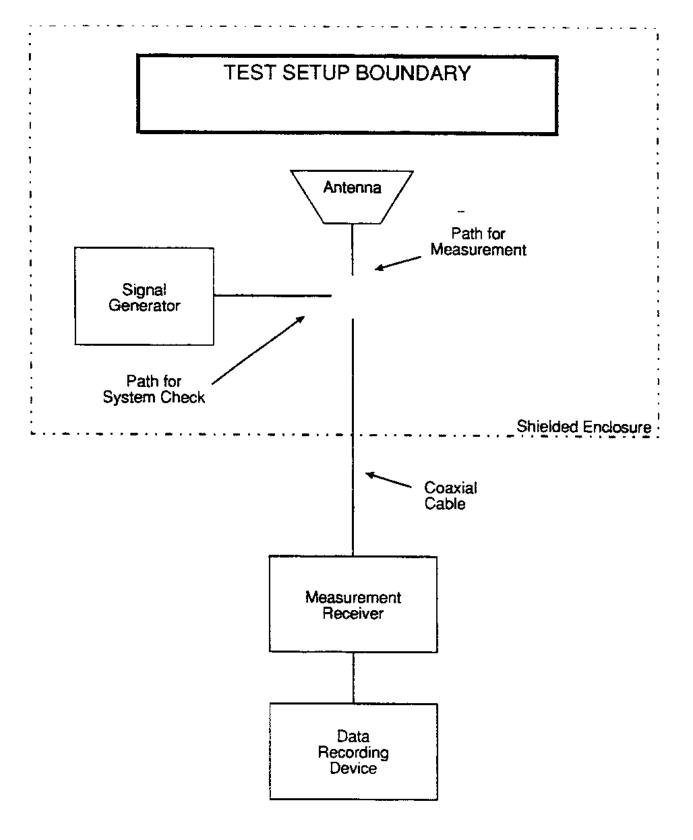
FIGURE RE102-1. Basic test setup.
