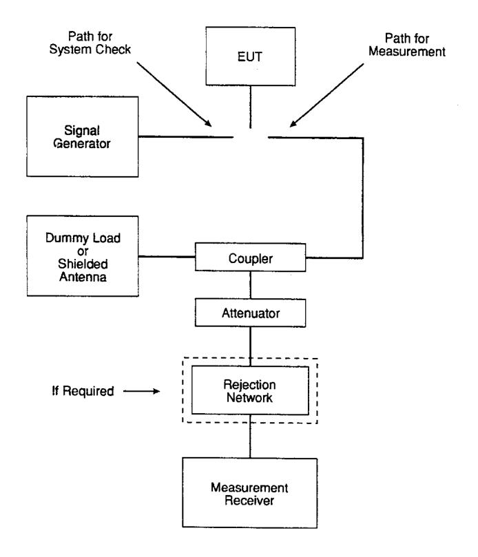
FIGURE CE106-2. Setup for high power transmitter.
