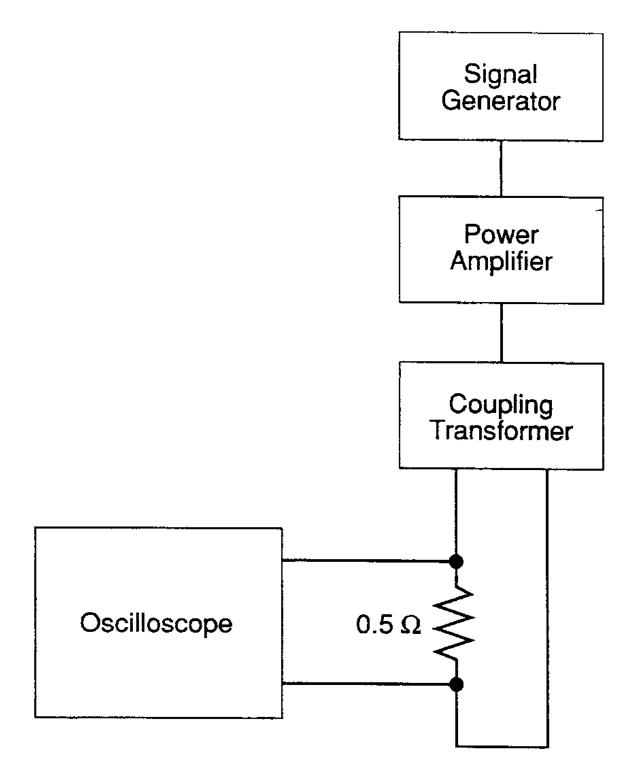
FIGURE CS101-1. Calibration.
