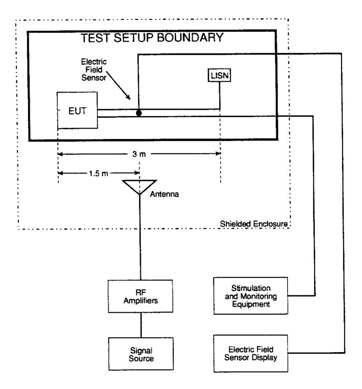
FIGURE RS103-1. Test equipment configuration.
