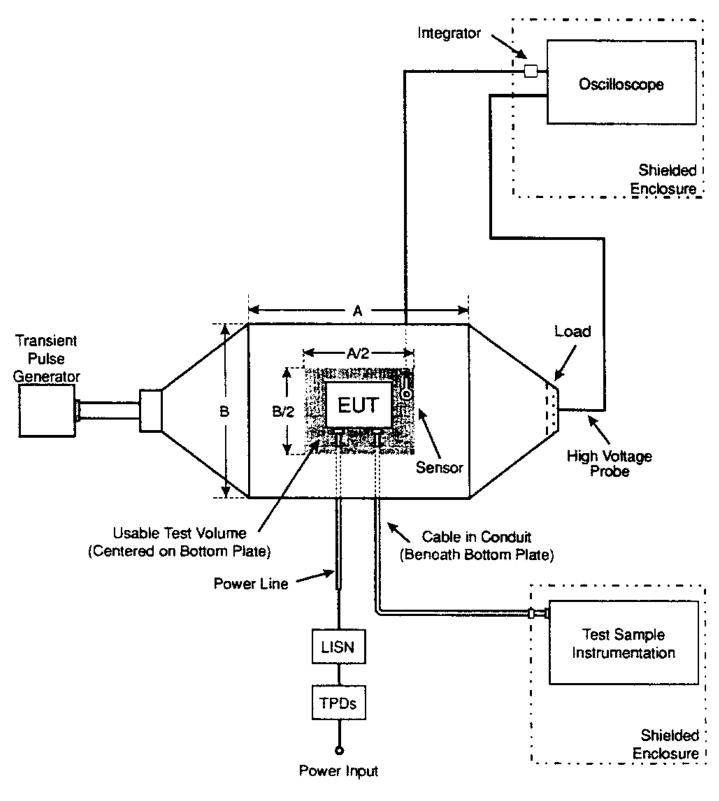
FIGURE RS105-2. <u>Typical test setup using parallel plate</u> radiation system.
