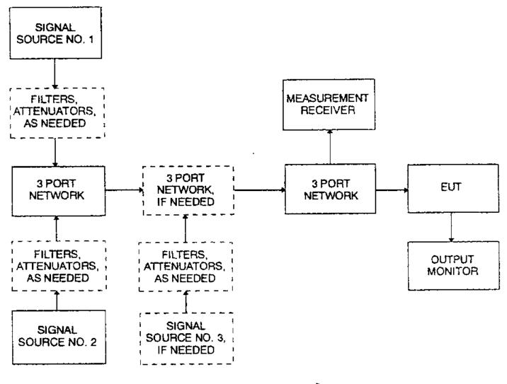
FIGURE A-5. CS103 General test setup.
