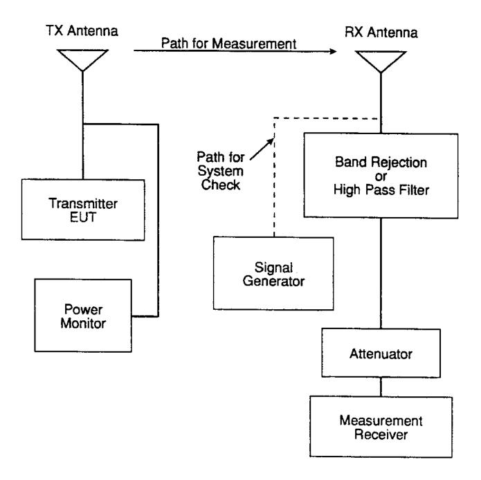
FIGURE RE103-1. <u>Calibration and test setup for radiated</u> <u>harmonics and spurious emissions, 10 kHz</u> to 1 GHz.
