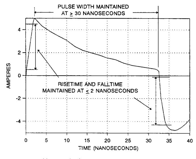
FIGURE A-11. Typical CS115 calibration fixture waveform.
