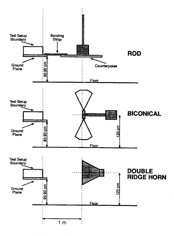
FIGURE RE102-2. Antenna positioning.
