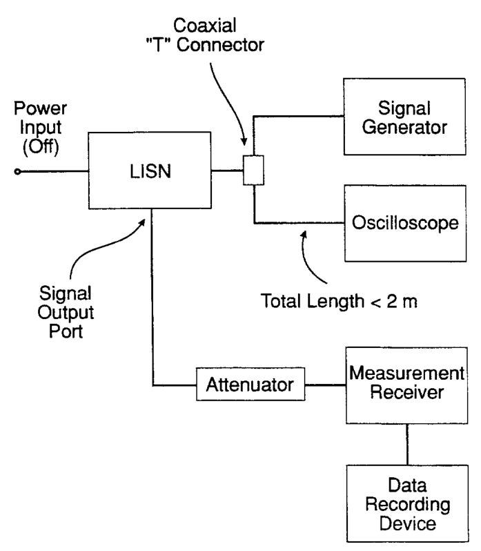
FIGURE CE102-1. Measurement system check setup.
