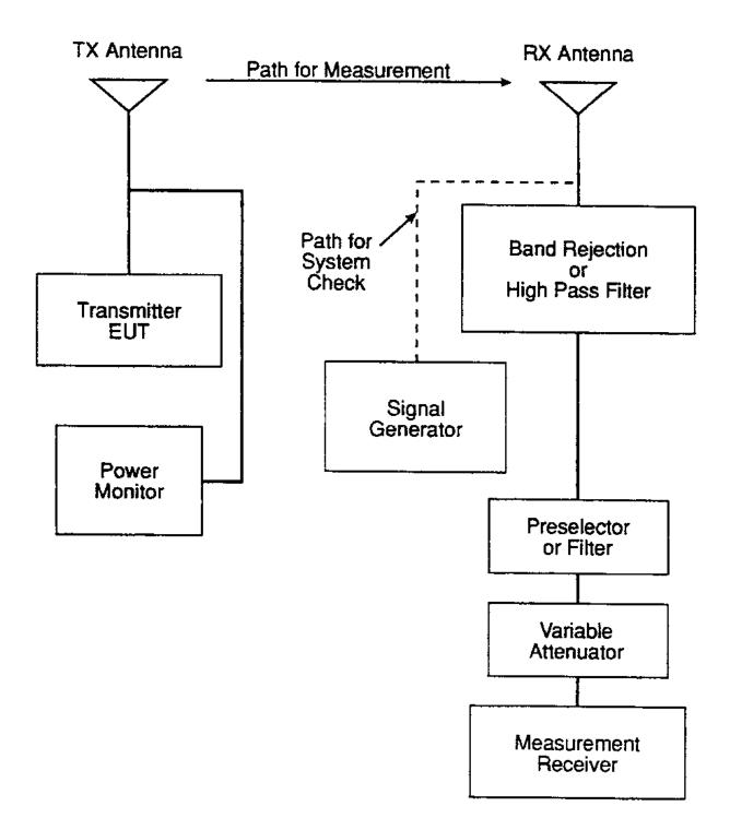
FIGURE RE103-2. <u>Calibration and test setup for radiated</u> <u>harmonics and spurious emissions, 1 GHz</u> <u>to 40 GHz</u>.
