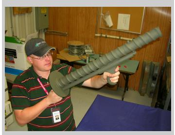
The HE-238-165-HH is a hand held directional antenna. The antenna is constructed entirely of aircraft certified 6061-T6 aluminum and G-10 fiberglass with copper radiator in a 100% sealed radome. This antenna was custom matched from 1.2 to 1.6 GHz to have the lowest VSWR possible, achieving a 2: 1VSWR across the band. The antenna is designed to provide many years of service.
