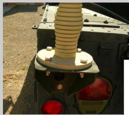
Using standard tools, the BM-03MM can be easily mounted and connected to an HMMWV within minutes.
