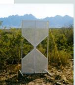
communications band (30 to 88 MHz) without the need for tuning systems. This rugged antenna is easily shipped/stored and can be set up and operational within a matter of minutes.
