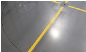
The gap between the floor and turntable can strictly be set de- pending on the performance of the anechoic chambers.
