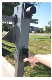
Support the mounting arm and loosen the lower vertical positioning screw. The mounting arm is released.
