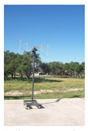
6. The antenna mounted on the mast in a 3m position.
