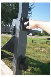
The positioning gimbal secures the mounting arm to the mast.
