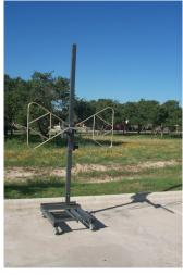
1. Antenna mounted on mast in lower position.
