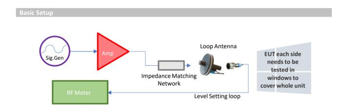
**Schlöder** has created a system to match this requirement. The system is computer-controlled to set the field level and perform testing with report generation.
