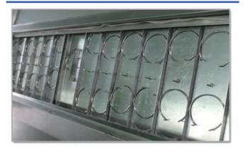
Standard sample holder can be adjusted to any thickness,test samples no need tocut to accommodate close range.
