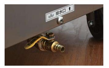
The bottom of the device is provided with drain cleaning tank to facilitate the drainage
