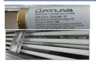
The UV lamp using ATLAS, spectral power distribution (SPD) will not change witht he lamp aging and longer life
