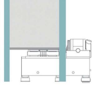
Vibration test systems and test chamber connect through table
