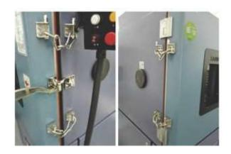
Using Explosion-proof lock and 2 Explosion-proof chains on each side for double protection.
