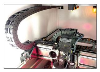
Figure 3: Flex cables on a robotic arm
