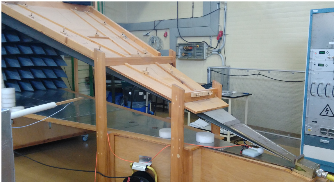
Figure 1: GTEM wave guide and pulse generator
